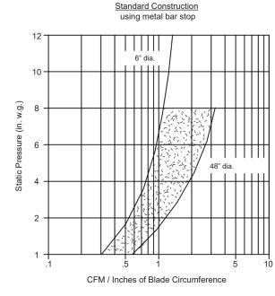
Leakage results shown are based on tests using various damper sizes. The shaded area between the graph lines indicate normal expected leakage range for a standard damper operating conditions and sizes.
